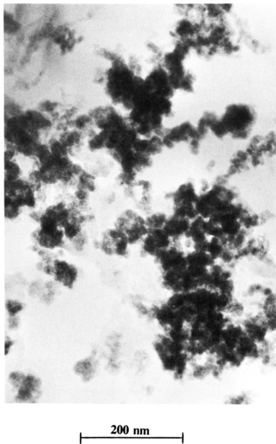
Figure 3. TEM micrograph of passivated Fe-Mg powders heat processed at 180 °C.
